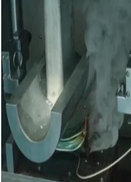
Lithium iron phosphate battery (extruded smoke)
