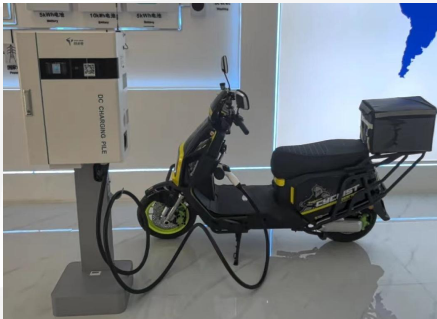
Nine-hole DC charging pile
